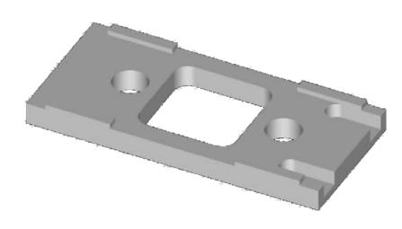
(\$cutout 2) (\$thru-round-hole-04) (\$closed-pocket 0) (\$blind-round-hole-0 0) (\$rectangular-cutout 0) (\$closed-rectangular-pocket 0) (\$boss 4) (\$rectangular-boss 4) (\$open-pocket 2))
