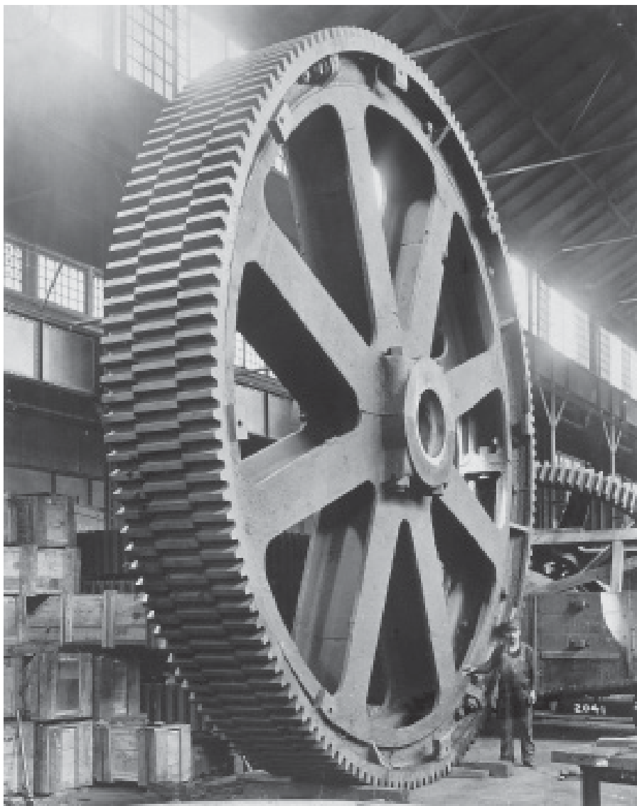
Molded staggered tooth gear and worker from the Mesta Engineering Company. A grant to the University of Pittsburgh helped to preserve records in the Archives of American Industrial Society.
