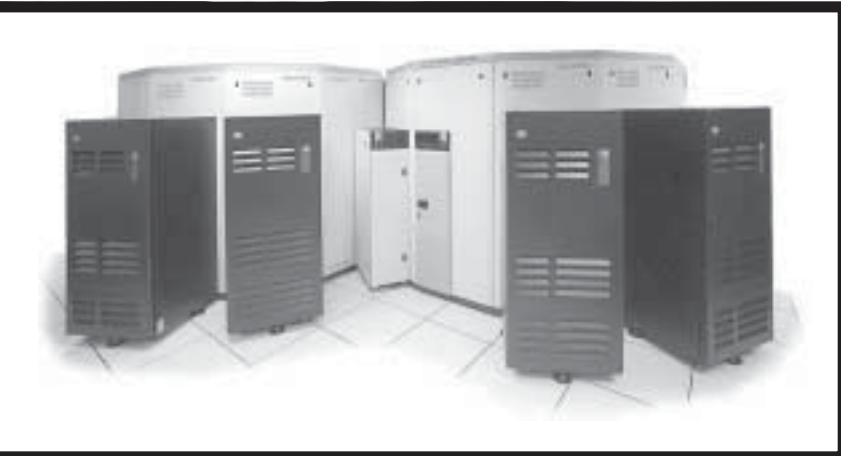
Two of the three StorageTek 9310 tape silos at SDSC. Each silo holds up to 6,000 tapes, and each tape can hold up to 20 GB of data. (Courtesy, SDSC)
